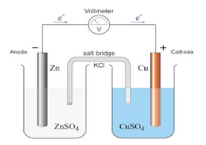
**CONSTRUCTION**: A` galvanic cell consist of the following parts.
